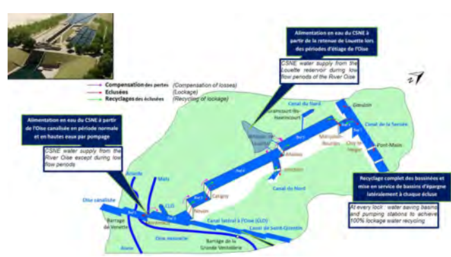
Fig. 14 Synopsis of the Seine-Nord Europe Canal and its water supply system, France; photomontage: illustration of a lock, with its water-saving basins and integrated pumping station, Q108-R9 [9]
