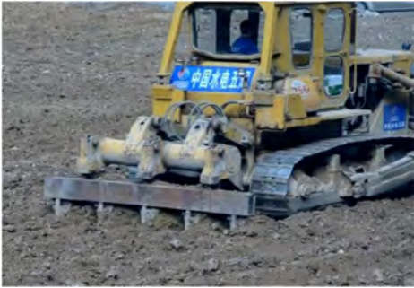
Fig. 7 Soil drying and paving equipment
