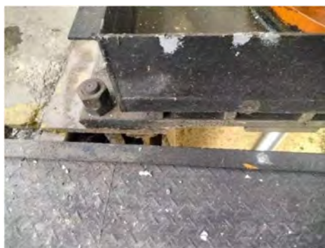
Fig. 4 Support base for the oil cylinders
