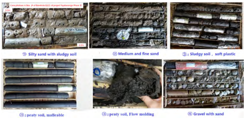
Fig. 3 Photograph of core samples of each soft soil layer drilling in riverbed
