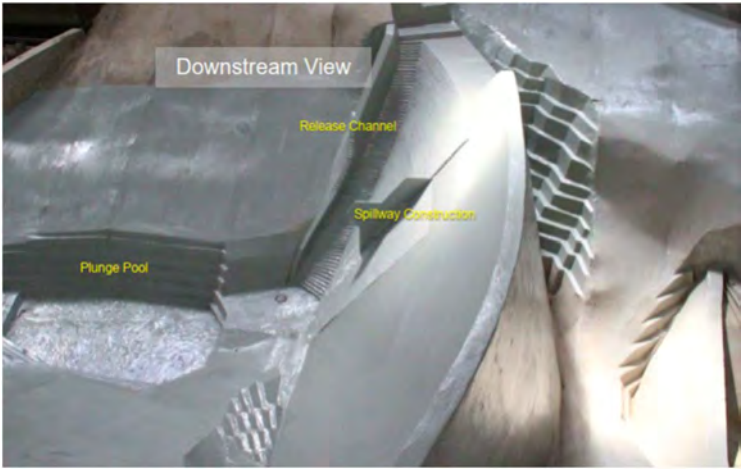
Fig. 5 Hydraulic Model for River Diversion Through the Dam Site in the 2021 Rainy Season
