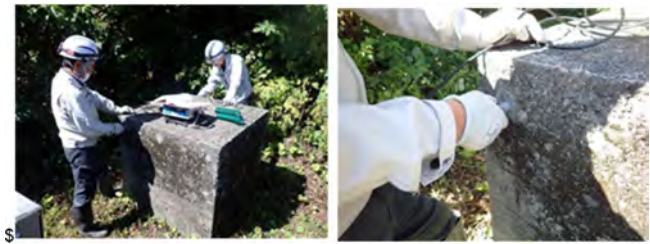
Fig. 6 Situation for monitoring ultrasonic wave propagation Situation de surveillance de la propagation des ondes ultrasonores
