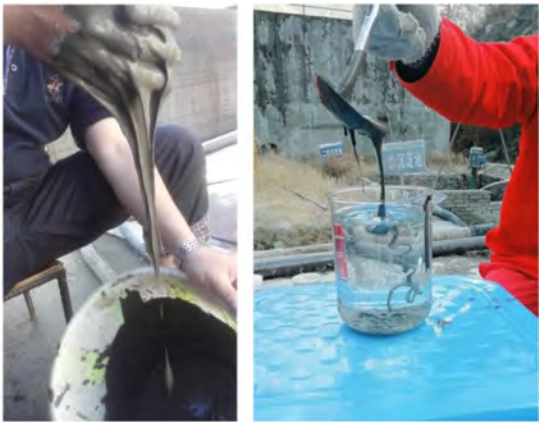
Fig. 4 HSPC non-dispersible underwater, Anti-Washout and rapid hardening grout paste
