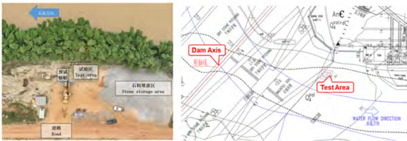
Fig. 5 Schematic diagram of the in-situ test area of stone column in dam foundation
