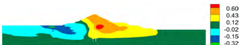
Fig. 13 The horizontal displacement after impoundment (Unit: m)
