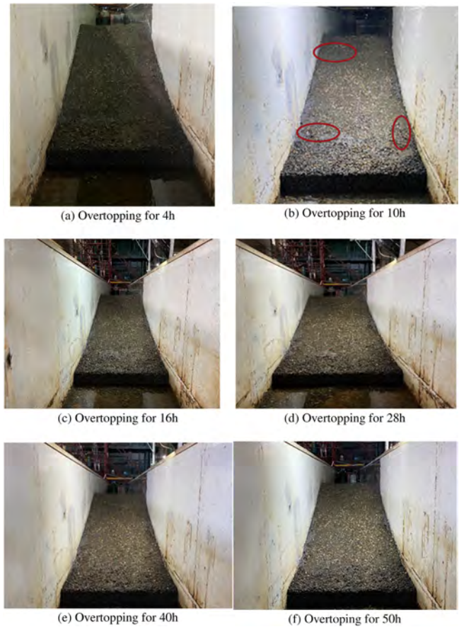
Fig. 8 The erosion of downstream surface under overtopping
