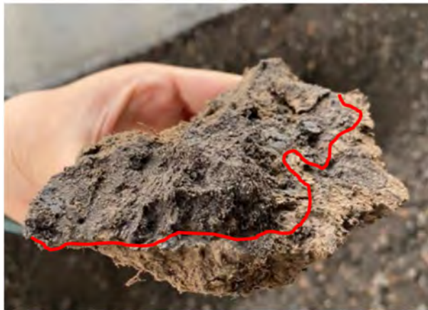
Fig. 10 The bonding between the embankment dam and reinforcement layer
