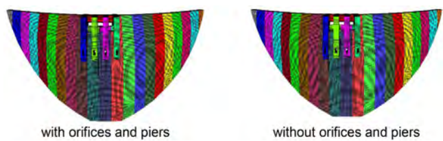
Fig. 2 The finite element meshes of the dams
